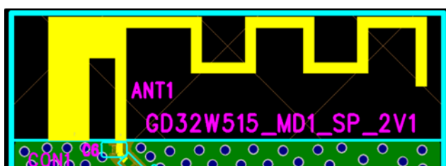
Figure 3-4. PCB antenna layout design
