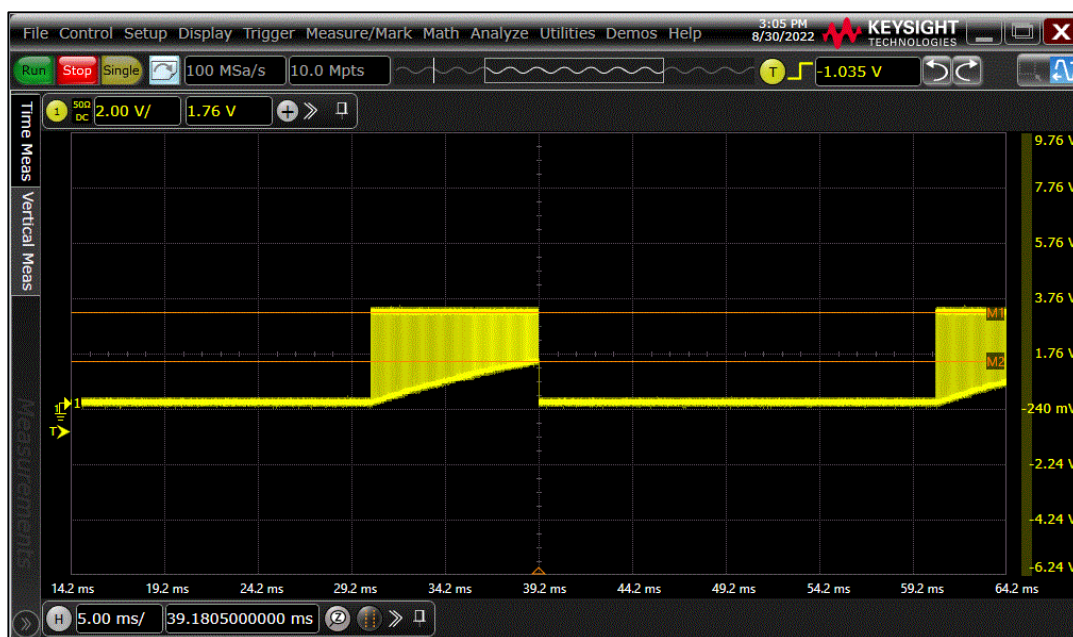
Figure 3-2. Channel pin charge transfer waveform
